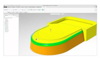
Apply draft to surfaces with adjacent rounds or chamfers. This example uses a round chain as the hinge.
